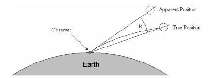
Figure 5.9 The apparent position of the celestial body is appeared to be higher than it's true position.
