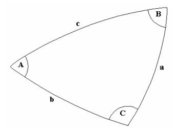
Figure 4.2 A spherical triangle.
