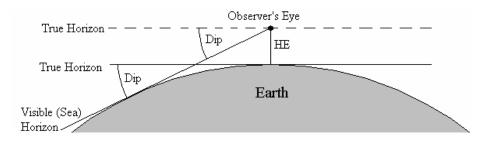
Figure 5.8 The visible sea horizon is dipped below the true horizon.
