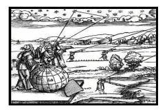
Figure 8.1 Lunar distance from a star is being measured with a cross-staff.
