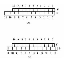
Figure 5.7 Vernier scale: showing subdivisions of a main scale.
